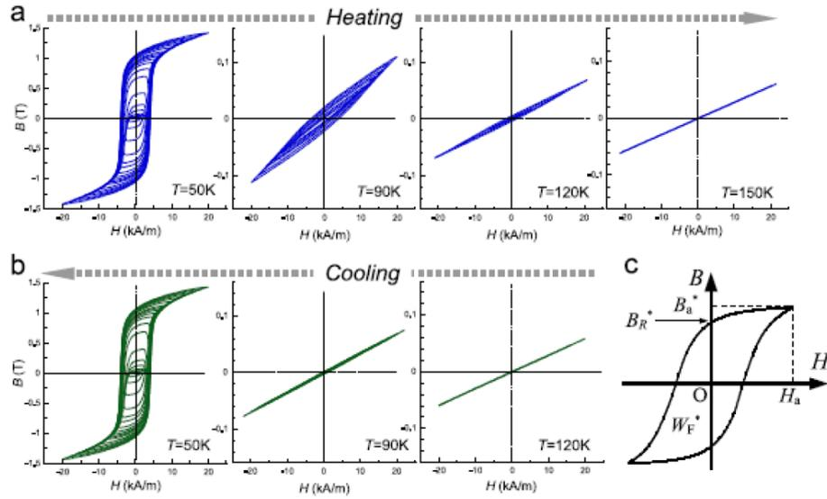
**Fig. 4.**  $B$ - $H$  hysteresis loops with different amplitudes of the magnetic field  $H$ , shown at different temperatures during (a) heating, (b) cooling; (c) the hysteresis loop parameters  $B_a^*$ ,  $B_R^*$  and  $W_F^*$  are the maximum flux density, remanent flux density and hysteresis losses, respectively. Reproduced from S. Kobayashi [29], with permission. Copyright (2011), American Physical Society, DOI: 10.1103/PhysRevLett.106.057207.
